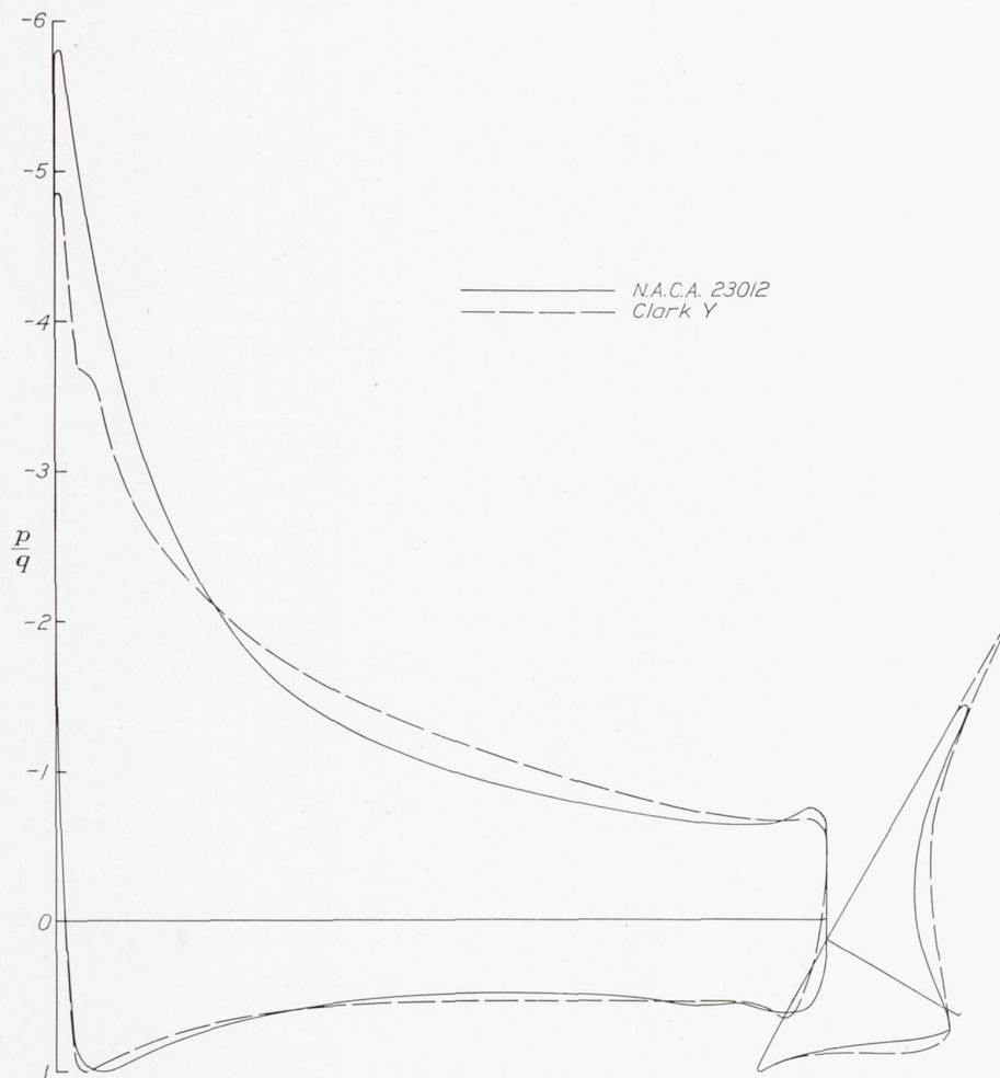
FIGURE 11.—Comparison of the pressure distribution, at the same lift, on the Clark Y airfoil and the 0.20c_w Clark Y Fowler flap with that on the N. A. C. A. 23012 airfoil and the 0.20c_w N. A. C. A. 23012 Fowler flap. c_{n(w+f)} = 2.35 .
