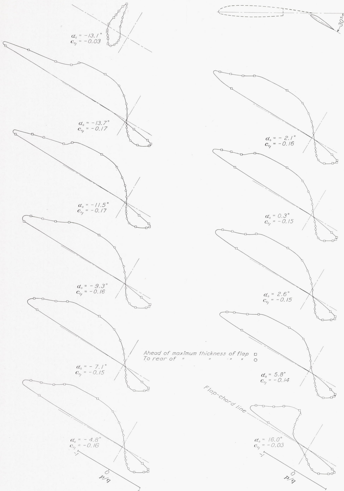
FIGURE 13.—Chord pressure distribution on the 0.30c w N. A. C. A. 23012 Fowler flap mounted on the N. A. C. A. 23012 airfoil. Flap deflected 30°.
