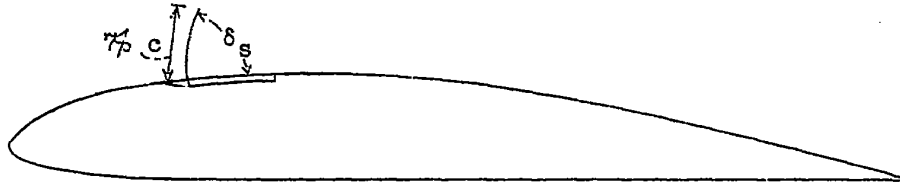
Plain Clark Y wing. Curved spoiler 7 per cent chord wide and 40 per cent semispan long.
