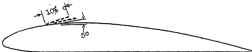
Plain Clark Y wing. Curved spoiler 10 per cent chord wide and 40 per cent semispan long, 5° deflection only.
