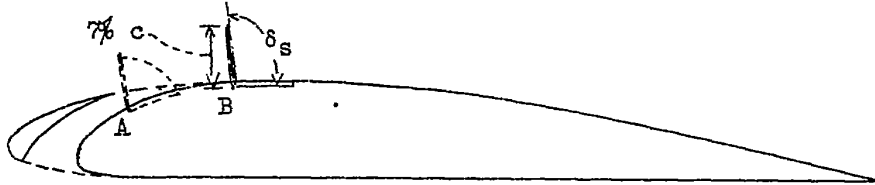
Clark Y wing with low-drag fixed tip slot 40 per cent semispan. Plain curved spoiler 7% c wide and 40 per cent b/2 long.
